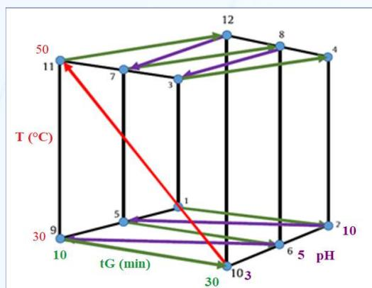
**Figure 2:** Automated experimental design (Design of Experiments, DoE) and conditions of tG-T-pH model. Twelve preliminary experiments were carried out with gradient range 55%  $\rightarrow$  90% eluent B (composition of eluent B was acetonitrile: THF = 7:3) and flow rate of 0.2 mL/min.
