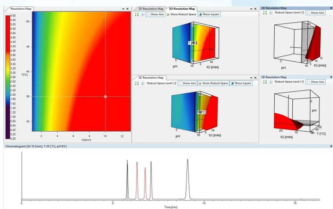
**Figure 3:** Visualization of the method operable region (MODR) and selection of the working point (column BEH C18 150 x 2.1 mm, 1.7  $\mu\text{m}$ , eluent A pH 9.5, column temperature  $T_C 35^\circ\text{C}$  and gradient time  $t_G 10 \text{ min}$ ).
