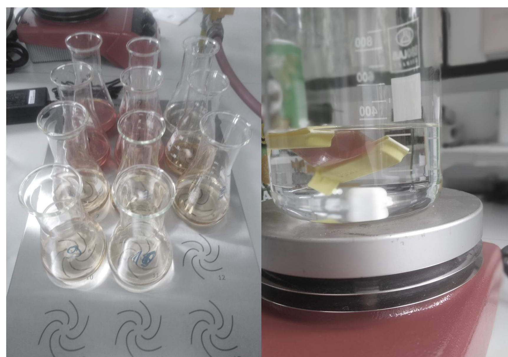
Figure 1. Chemical and biogenic synthesis (A) and purification by dialyzing tubing (B) of selenium nanoparticles
