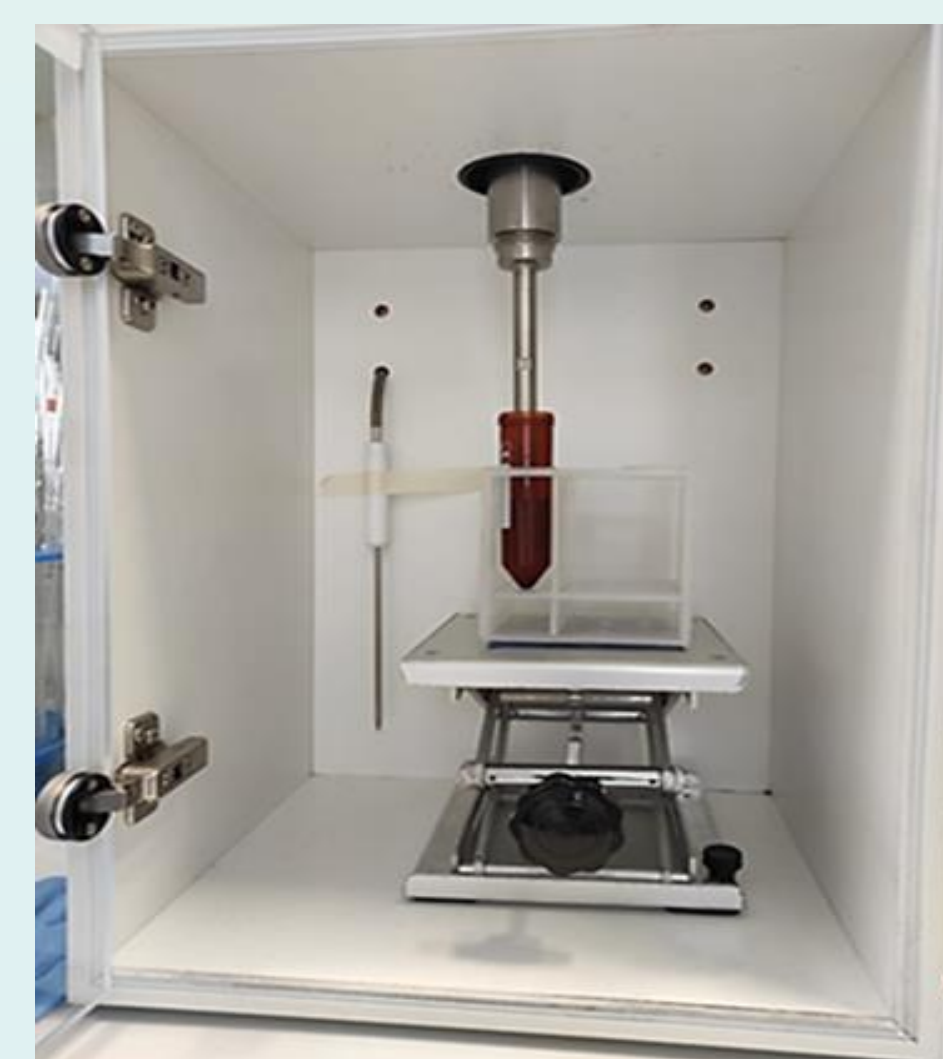
Figure 1. Apparatus for direct ultrasonic extraction (Sonoplus 3100, Bandelin, Berlin, Germany)
