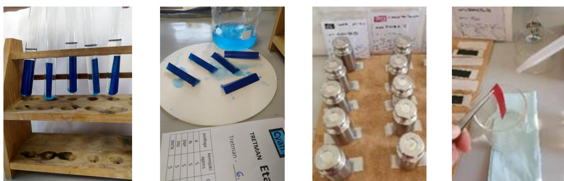
Figure 2. Chemical stability test with ethanol, acetic acid and sodium hydroxide
