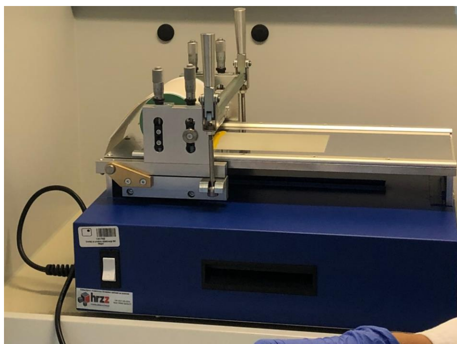
Figure 1. Printing with a laboratory device KPP Gravure system
