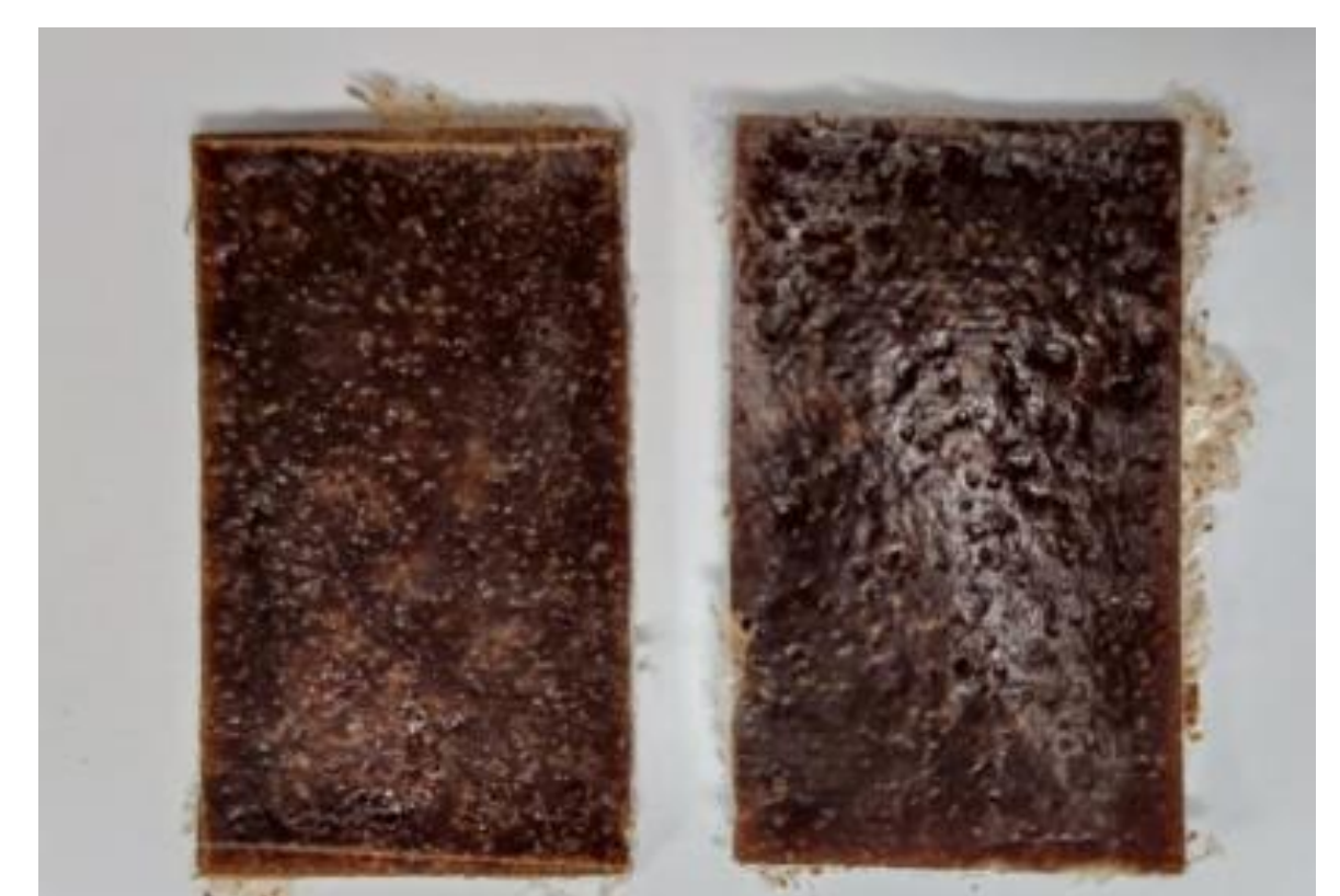
Figure 3. Tiles after pressing of PLA composites with 25 wt.% pepper seed cakes
