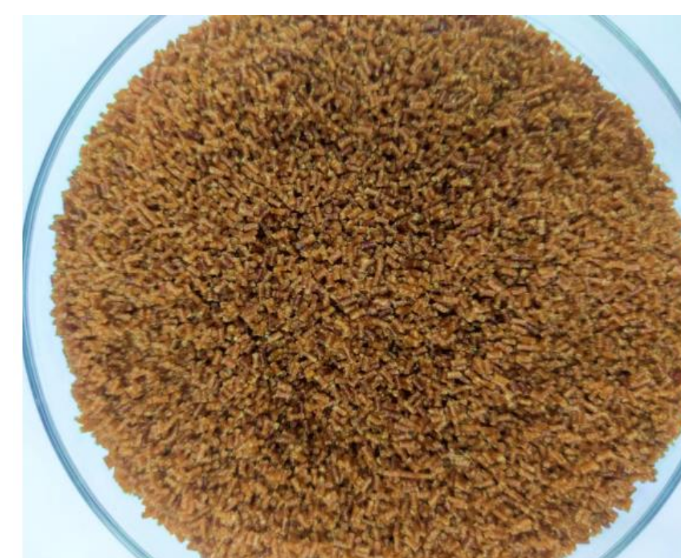
Figure 2. PLA composite with 25 wt.% pepper seed cakes
